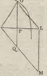
any perpendicular from the circumference upon KL, KP being x, OP will be y. Either of the points, therefore, in which these two loci intersect each other, as O, will give OP an ordinate in both equations, KP being the common absciss; therefore KP, OP are the two perpendiculars required, from which the point F is easily found.
